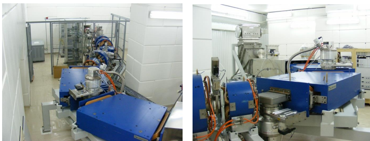
Fig. 1 Mass-spectrometer “MASHA” at the beam line of the cyclotron U-400M
