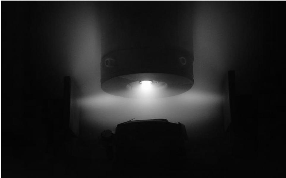
*Figure 2 Photography of DC pulse plasma jet system during  $TiO_x$  sputtering.*
